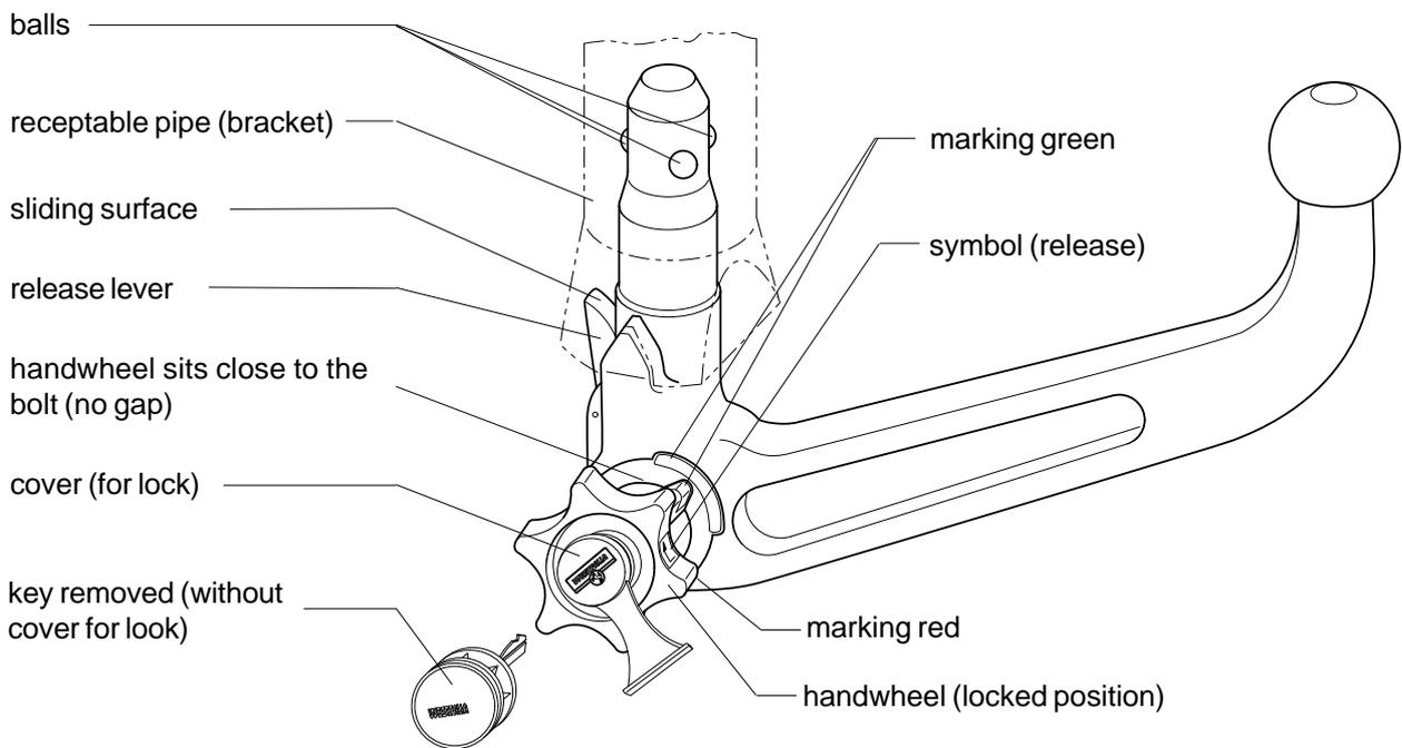
**Unlocked position (coupling hitch unmounted)**
