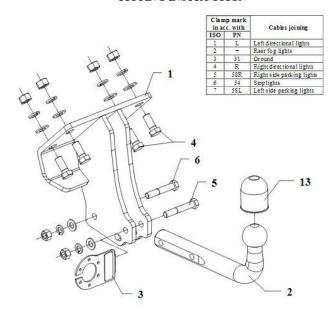
This towing hitch is designed to assembly in following cars: MERCEDES 230-300 GE, 250 - 300 GD produced since 1980 catalogue no. D25 and is prepared to tow trailers max total weight 3500 kg and max vertical mass 120 kg.
