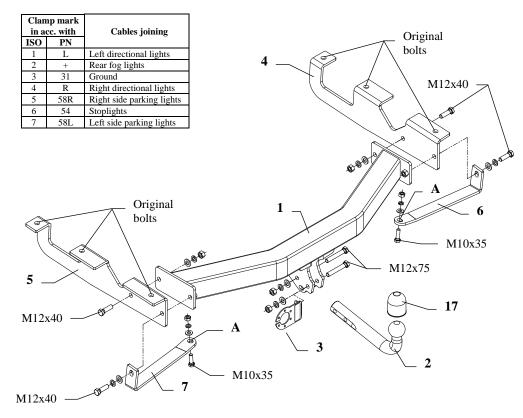
This towbar is designed to assembly in following cars: **JEEP GRAND CHEROKEE (WJ/WG)**, produced since 04.1999 till 05.2005, catalogue no. **JP04** and is prepared to tow trailers max total weight up to **3500 kg** and max vertical load **140 kg**.
