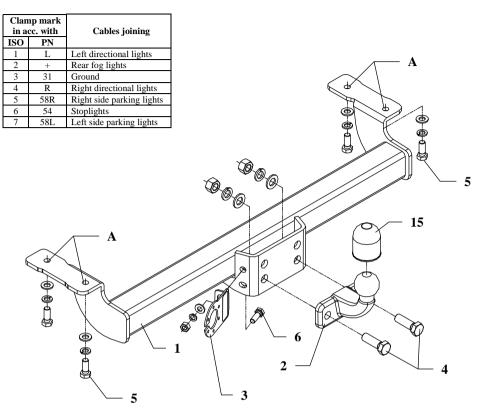
This towing hitch is designed to assembly in following cars: **SUZUKI VITARA, 5 door, spacing of holes in frame 820mm,** produced since 03.1995 till 08.1998, catalogue no. **W05** and is prepared to tow trailers max total weight **1875 kg** and max vertical load **75 kg**.
